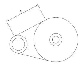
B. At the center of the span (K) apply a force (perpendicular to the span), large enough to deflect the belt 1/64" for every inch of span length.
