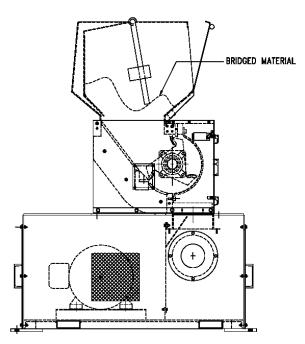
**BRIDGE/BRIDGING:** OCCURS WHEN MATERIAL BLOCKS ITS OWN FLOW AND DOES NOT FALL INTO THE <u>CUTTING CHAMBER.</u>
